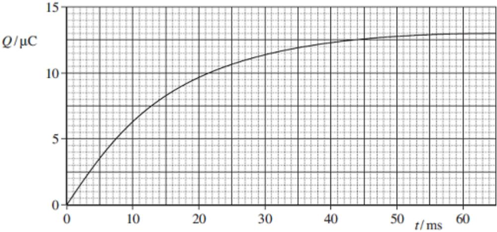
(b) (i) When the capacitor is fully charged, the charge stored is  $13.2 \mu\text{C}$ . The electromotive force (emf) of the battery is  $6.0 \text{ V}$ . Determine the capacitance of the capacitor.
