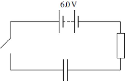
The switch in the circuit is closed at time  $t = 0$ . The graph shows how the charge  $Q$  stored by the capacitor varies with  $t$ .
