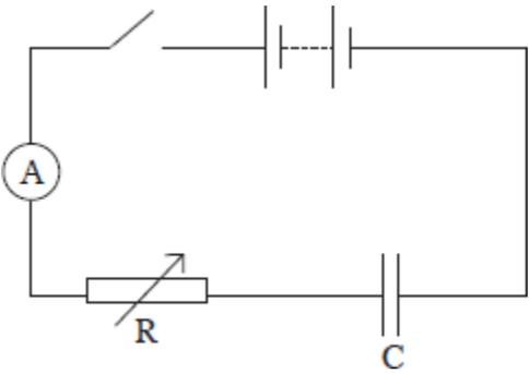
Calculate the resistance of  $R$  when the uncharged capacitor has been charging for  $30 \text{ s}$ .
